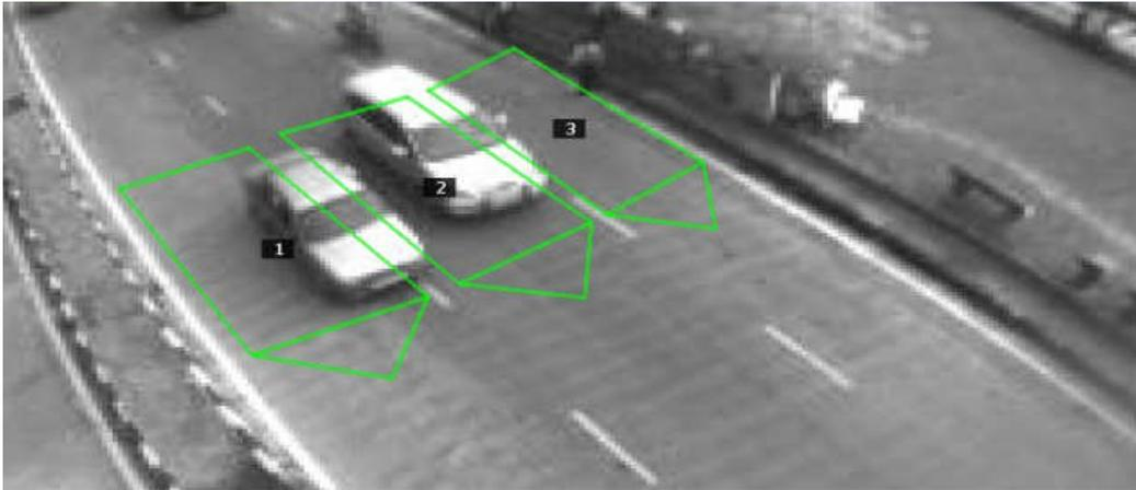
Outlined above is an illustration of this Marine Drive location of a typical video detector position and the associated configured zones of detection.
